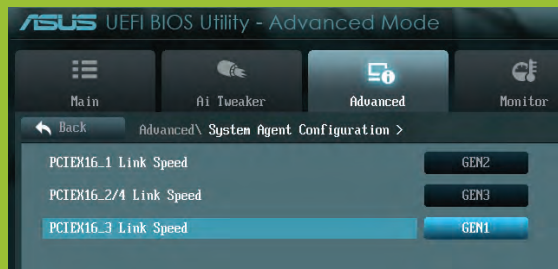
Our motherboard let us toggle between Gen 2.0 and Gen 3.0 easily, though X79 doesn't natively support Gen 3.0.
